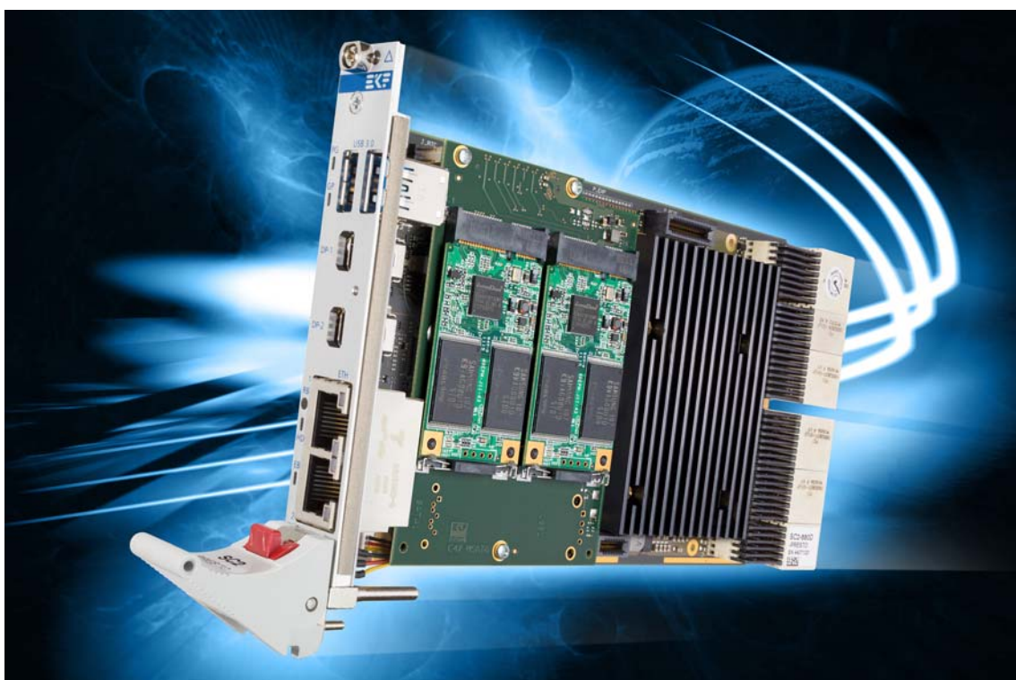
SC2-PRESTO w. C47-MSATA Mezzanine Module 4HP Assembly
