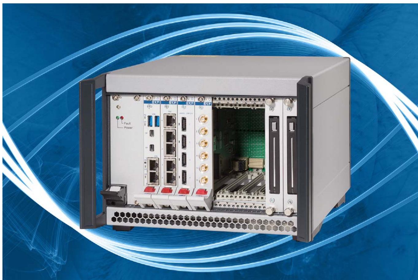
SRS-4401-RACK for up to 8 Peripheral Slot Cards
