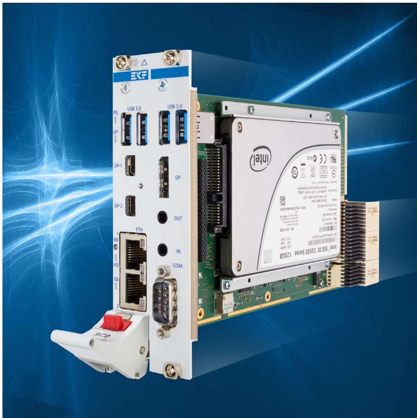
8HP Assembly SC2-PRESTO w. SCS-TRUMPET Mezzanine Side Card (2.5-Inch SATA SSD)
