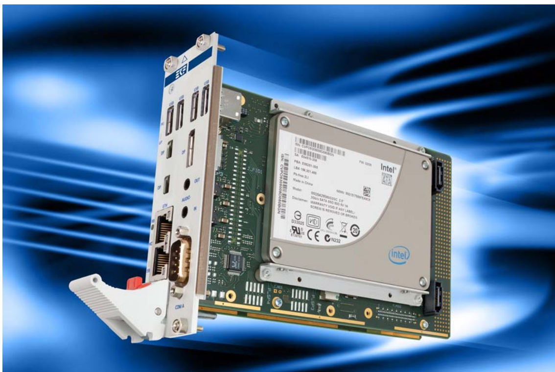
SC2-PRESTO w. PCS-BALLET Side Card & 2.5-Inch SSD, 8HP
