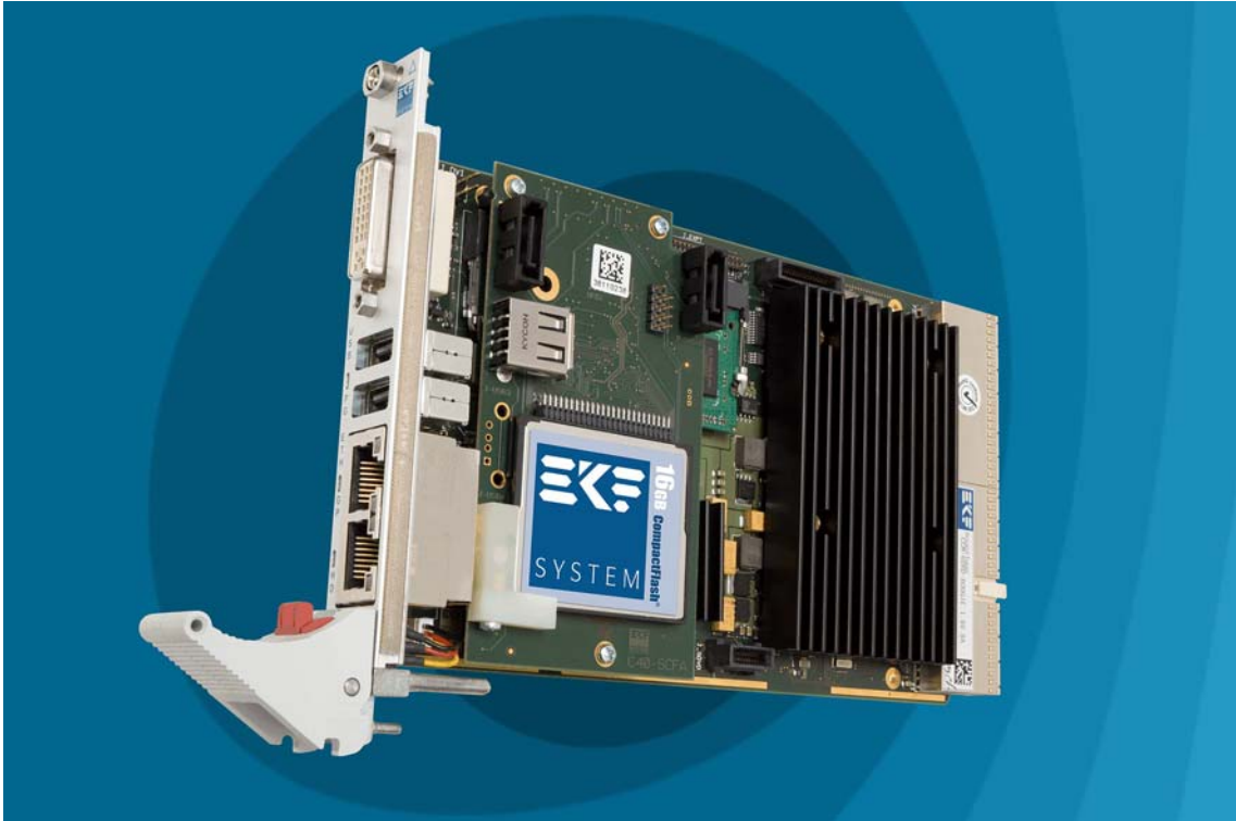
C40-SCFA (CF Card Version) on a CPU Carrier Board CCM-BOOGIE
