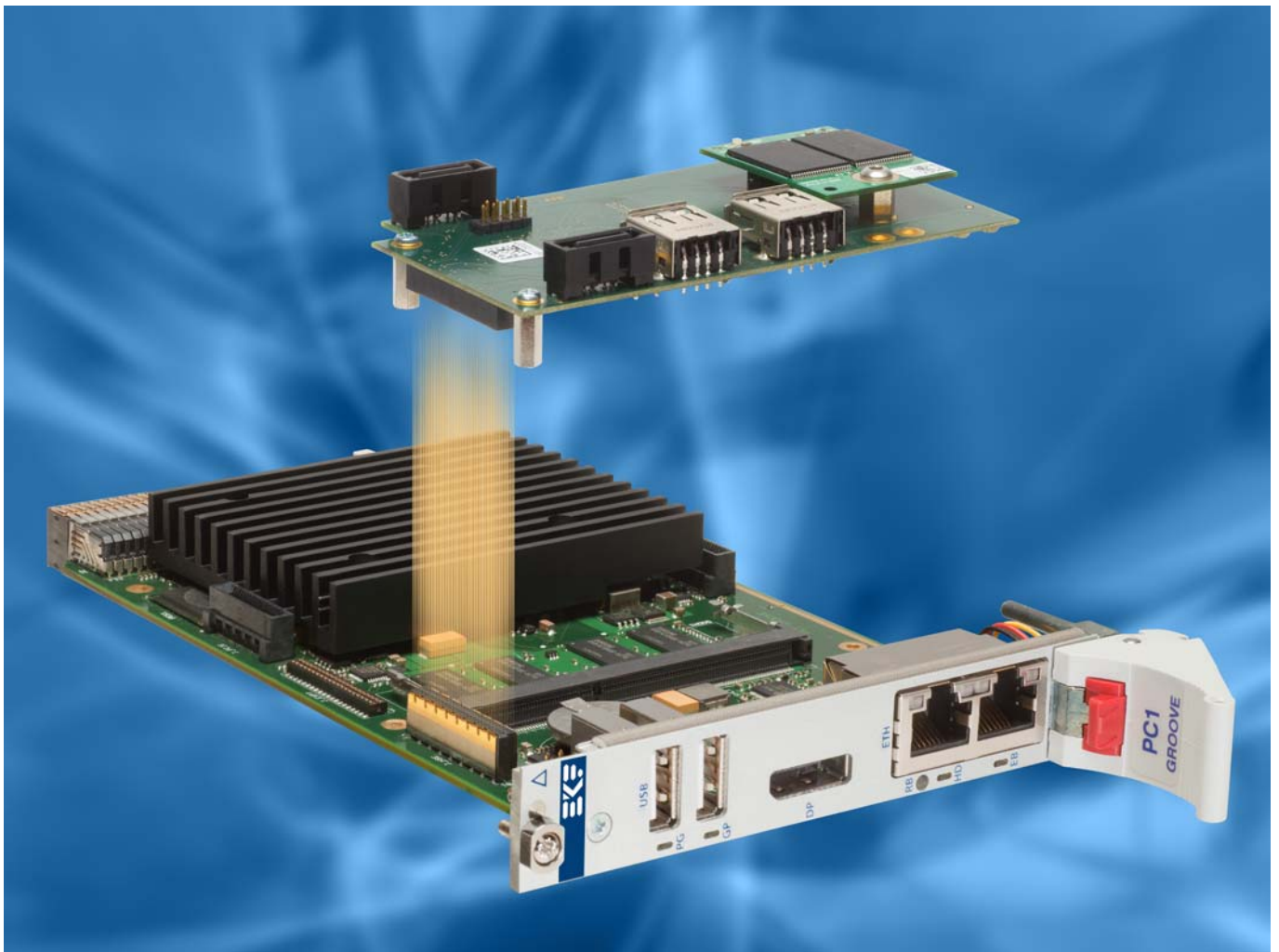
C40-SCFA (USB SSD) over PC1-GROOVE CPU Carrier Board
