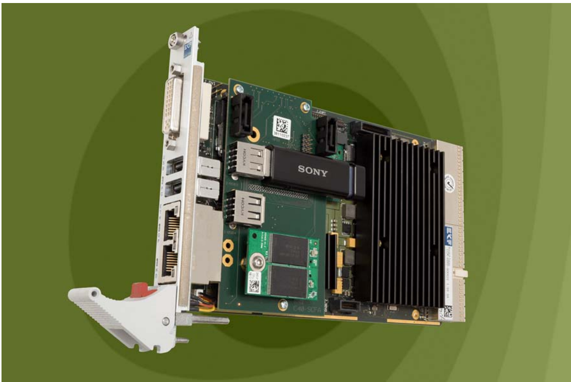
C40-SCFA (USB SSD Module Version) on the CCM-BOOGIE
