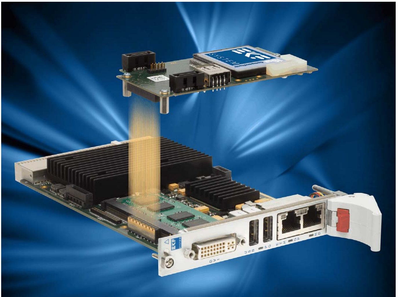
C40-SCFA (CF Card) over CCM-BOOGIE CPU Carrier Card
