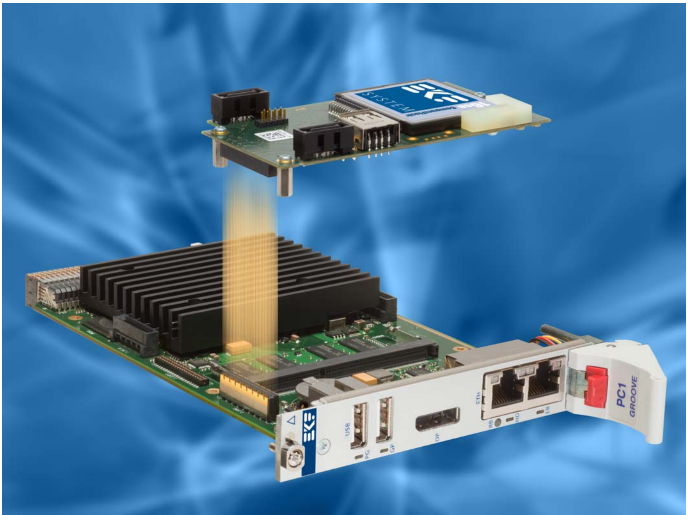
C40-SCFA (CF Card) over PC1-GROOVE CPU Carrier Board
