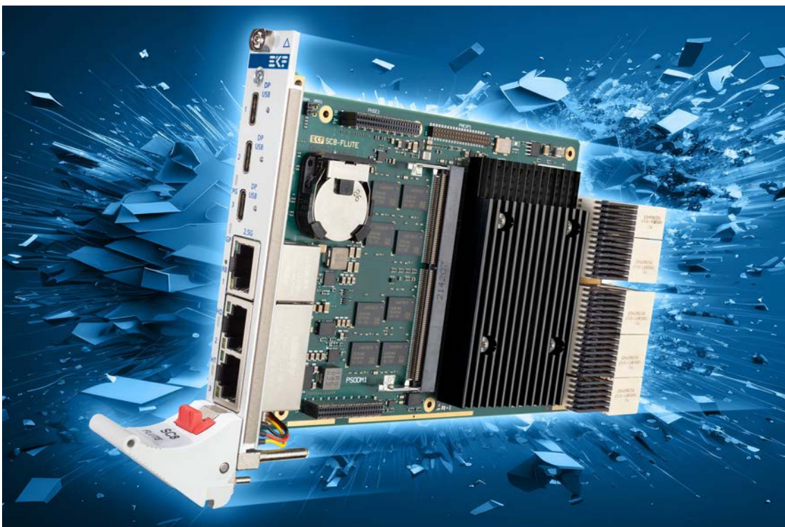
SC8-FLUTE - Soldered RAM Top/Bottom
