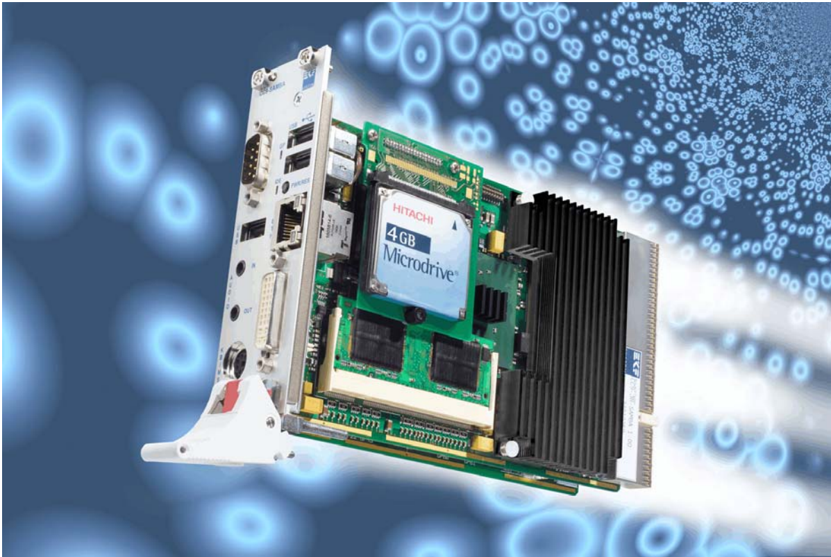
CCA-LAMBADA Mounted on Bottom of CC9-SAMBA
