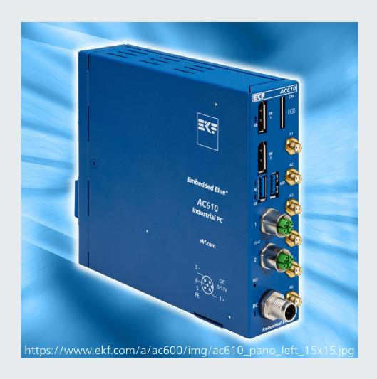
As a member of their **Embedded Blue®** DIN Rail series, **EKF** presents the **AC610**, a fully featured industrial PC. Equipped with an Intel® E39xx (Apollo Lake-I) processor, and offers two connectors each for DisplayPort monitors, USB3 and M12-X Gigabit Ethernet at the front.
